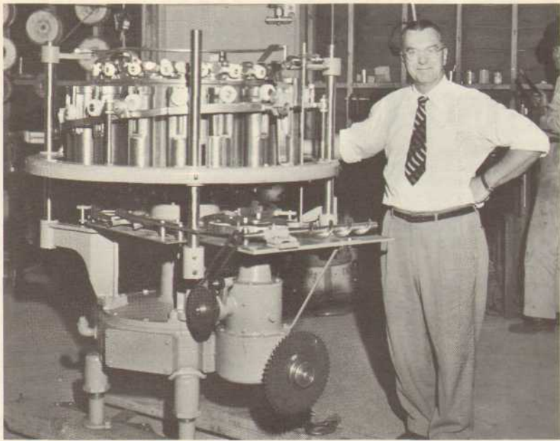
EVERETT MINARD , Santa Ana Division engineer, poses with his latest creation, an 18-station food filler built for Campbell Soup. An even larger unit, the 36-station filler shown in production elsewhere on the page, will be ready for delivery in the near future.
