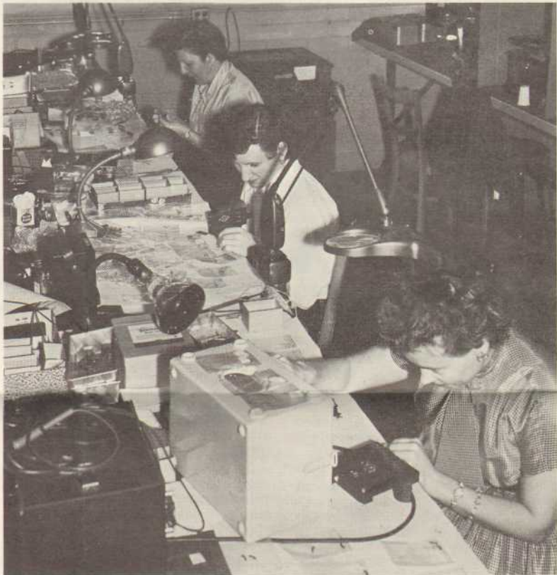
ASSEMBLY OF READ —Record heads used in the LGP-30 is performed by (front to rear) Hedy Galyon, Retha Chism and Grace Vessella. These sensitive devices pick up and record "bits" of digital data on a magnetic memory drum.
