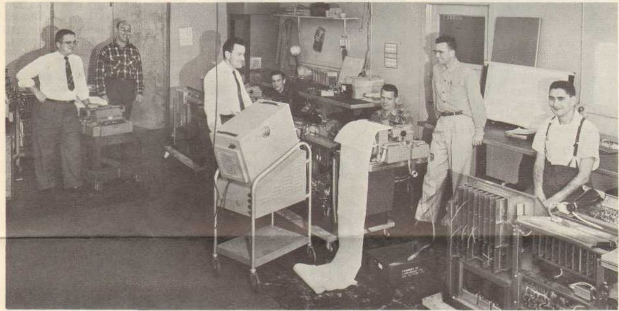
AFTER ASSEMBLY comes checkout, an exacting task that requires patience and a good deal of skill and experience. The men responsible for this phase of LGP-30 production include (l. to r.) Dick Wil-
