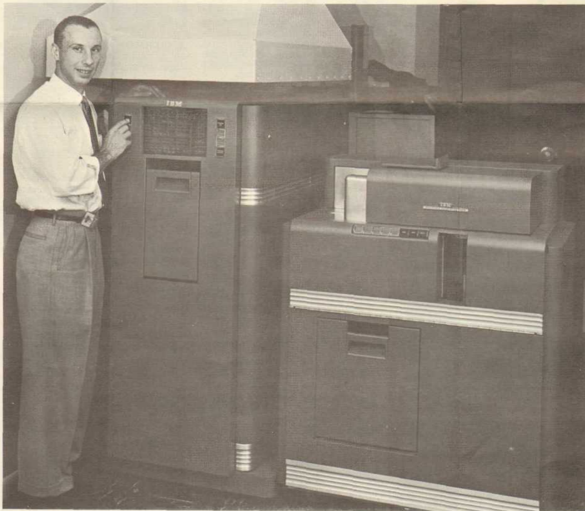
NEW CALCULATOR —Pete Mobley, IBM facility supervisor, is set to push the button that will set the completely electronic 604 Calculator in operation. This machine operates many times faster than
