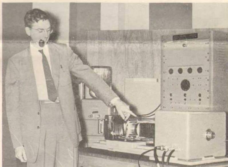
IMAGE CONVERTER —R. Carroll Maninger, PTI department director, points out the image converter tube used in the ultra-high speed electronic camera developed by Precision Technology for the University of California's Radiation Laboratory at a recent meeting of the Society of Motion Picture and Television Engineers in San Francisco. (Photo courtesy of PTI)
