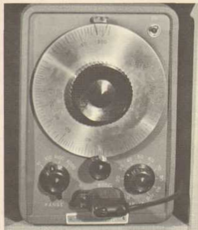
This oscillator varies the pitch of the sound, is also used to check child's hearing aid.
