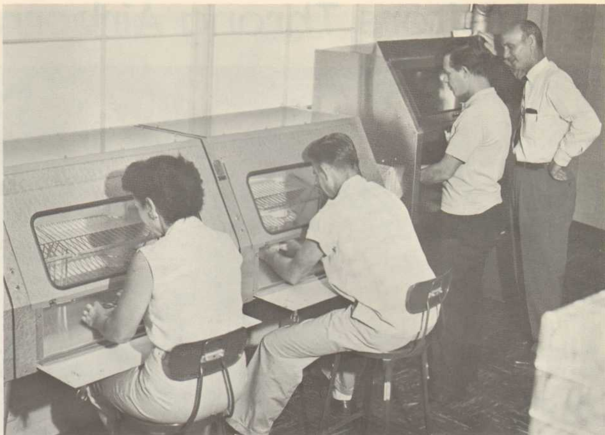
NEW DUST-FREE set up for assembly of intricate mechanisms is shown in new Providencia street plant in Burbank, which went into operation this month. General Foreman Max Schirmer (R), watches, (from right to left) Alex Janos, operating sonic cleaner, and Charles E. Morgan and Lorraine Mackey using dust-
