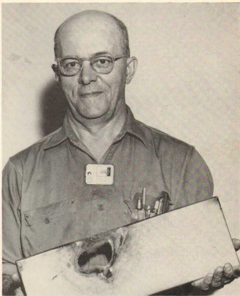
"A CLOSE CALL"—says Joe Buteau examining the results of an electrical explosion that sprayed molten metal on his hat and glasses. He holds the panel that made contact with the "hot" buss bar, showing where the heat burned a hole.
