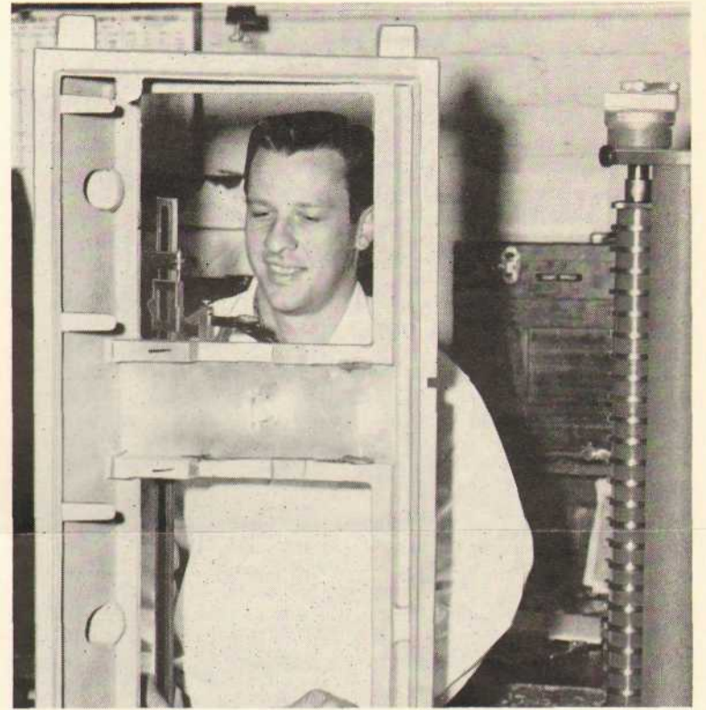
MILLING CHECK —Inspection of in-process work is a prime and exacting function of Quality Control. Ted Cherry, surface plate inspector, checks the milling of a computer panel cover with a plate check gage. The gage is one of numerous devices used for inspection.
