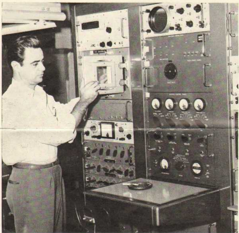
RECEIVING INSPECTION —Serge Diloires, precision electrical lead man, inserts a tachometer into the temperature chamber of a tachometer test stand, located in Bldg. 1. The tachometer, supplied by one of Librascope's many vendors, is given a functional test at 75 degrees C. All incoming materials are inspected by Quality Control.
