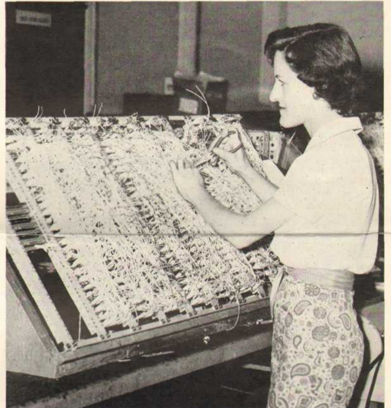
COMPLEX BUSINESS —The maze of wiring on a computer matrix is systematically checked by Quality Control. Typical of the matrices inspected is an ASROC matrix section, shown above. Irene Pekarick, general assembler, is doing the wiring.
