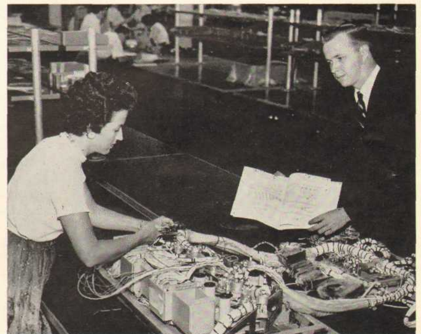
WIRING TECHNIQUES — are outlined in the Wireman's Workmanship Manual, developed by Engineering Standards. Leonard Novin (r), standards coordinator, goes over a standard technique with Lynne Adams, wireman, as she works on a SUBROC leveling computer.
