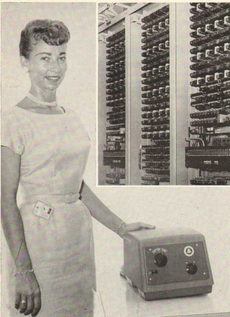
SOMETHING NEW in Librascope's modern telephone system is a "toll-diverter." When a number is dialed beyond the authorized Los Angeles toll area, the "toll-diverter" automatically cuts in a recording of PBX Supervisor Audrey Blythe, indicating an unauthorized call is being made. Audrey is shown here with the recorder. The complex diverter equipment is pictured in the inset.
