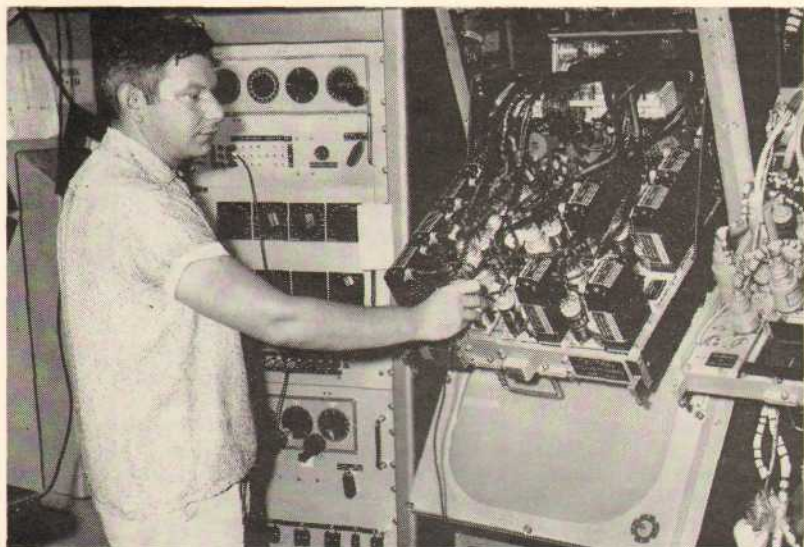
ASROC ADJUSTMENT —Instrument technician John Goad, Final Adjustment, is shown zeroing a converter on the Mk-38 during final test.
