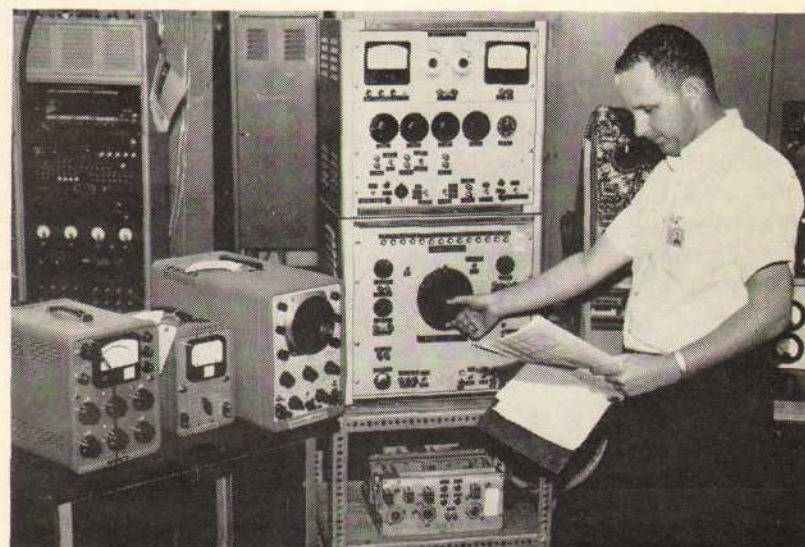
TESTING CP-209 —Instrument Technician Bob Holcomb is seen checking and certifying the CP-209 computer, using the FATS checkout book.
