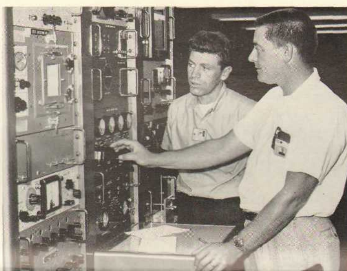
FINAL CHECK —Test Equipment Technician Dick Goetsch (r), discusses operation of the Tachometer Generator Test Station with Archie Darezzo, Incoming Inspection. The "tach stand" is the final test for high accuracy induction tachometers and servomotors.
