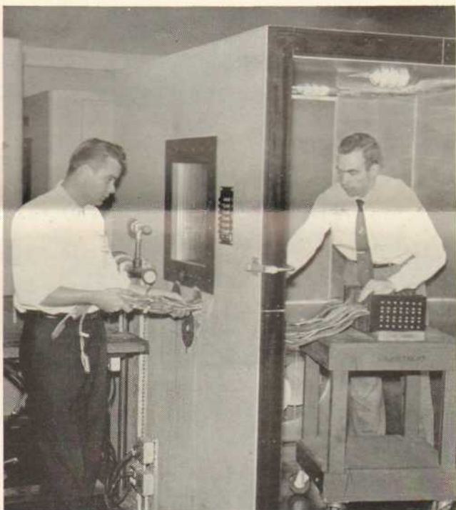
READY FOR TEST—Senior environmental technicians Dick Piety (left) and Frank Haskins are seen preparing a humidity test on diodes in Reliability humidity chamber.
