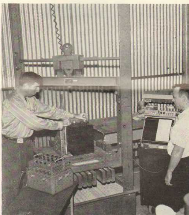
SECURING FOR SHOCK—Aerospace engineer Bob Hohenstein (left) and Reliability technician Jack Cooper are seen instrumenting for shock test on Aerospace computer ASN-24. During testing, it will be dropped from varying heights into the box of sand as a simulation of environmental conditions.
