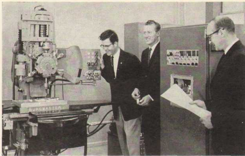
NEW EQUIPMENT —Manufacturing Planning Supervisor Ivan Franklin (left), and Industrial Engineers Jack Leighton and Chuck Keesling inspect the new, numerically controlled Burgmaster turret drill press and the Hughes positioning controls. The new equipment was delivered and installed early this month.
