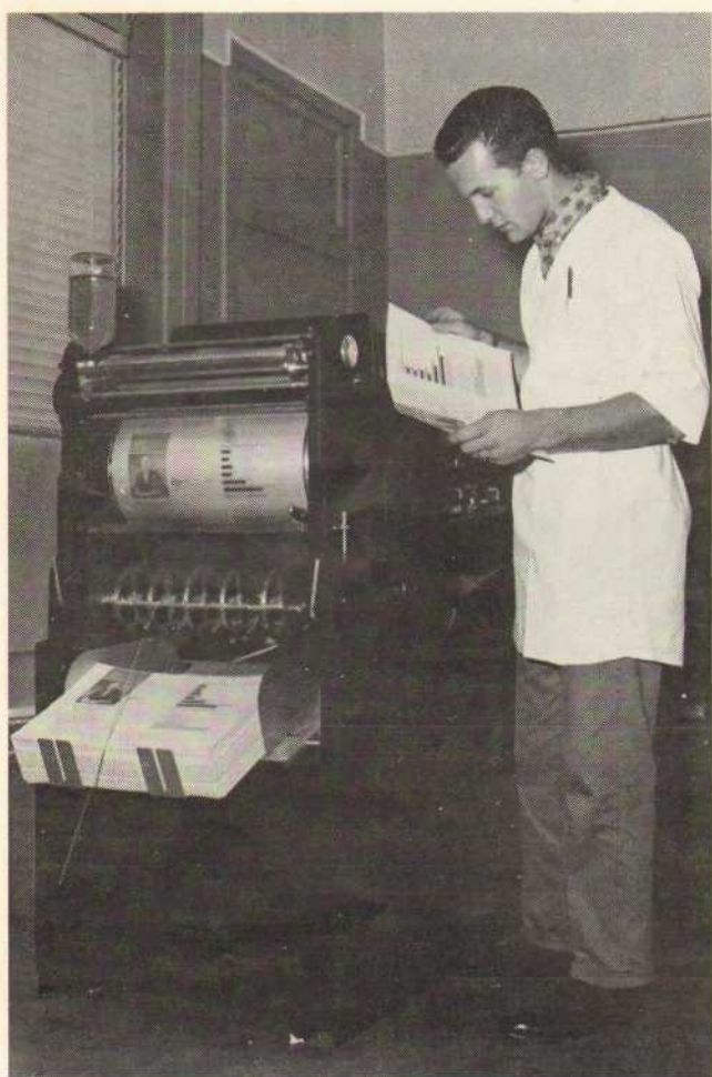
TIMELY DEBUT —Latest equipment to be added at Reproduction Services is this new offset printing press. Its first job—printing the 1960 Annual Report. Here, Ken Mandeville inspects sample of the product. The new press, which can handle pages up to 11 by 17 inches, offers expanded capabilities in printing for the section.
