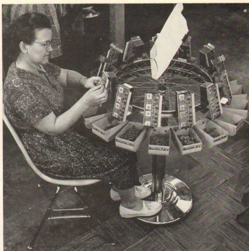
WHEEL OF PROGRESS —A working model of the "lazy-susan" assembly station, designed by Methods Improvement Group to cut component mounting time on circuit boards, is put through its paces by Electrical Assembler Mary Jane Jesse. Proposed for use in the Glendale Branch Processing, Wiring and Assembly Bldg. A-19, the rotary device would replace present bench assembly methods.
