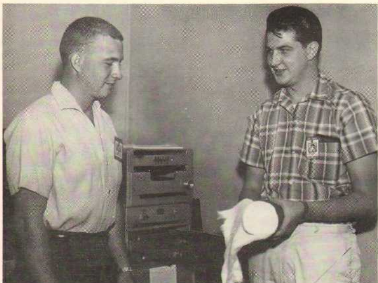
POWDER FOR PRINTING —The Zerox camera process, handled by Jerry Schweigert (left) and Don Brown, produces the Master Sheets for each page to be printed. In the process, fine powder clings to an electrically-charged plate corresponding to each line or character on the original paper. After a trip through the Zerox oven, the powder becomes a permanent, hard grease which, in offset printing, is the equivalent to pieces of type used in other processes.
