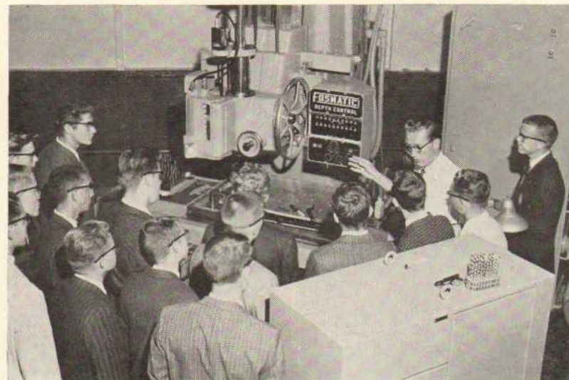
HOW IT WORKS—Industrial Engineer Jack Leighton (on right), explains "numerically controlled" Fostick Jig Borer to touring group of high school students, during recent annual Boys' Week observance. All of the students, incidentally, aren't suffering from faulty vision. Following Librascope safety practices, each visitor was outfitted with a pair of safety glasses while touring the shop areas.
