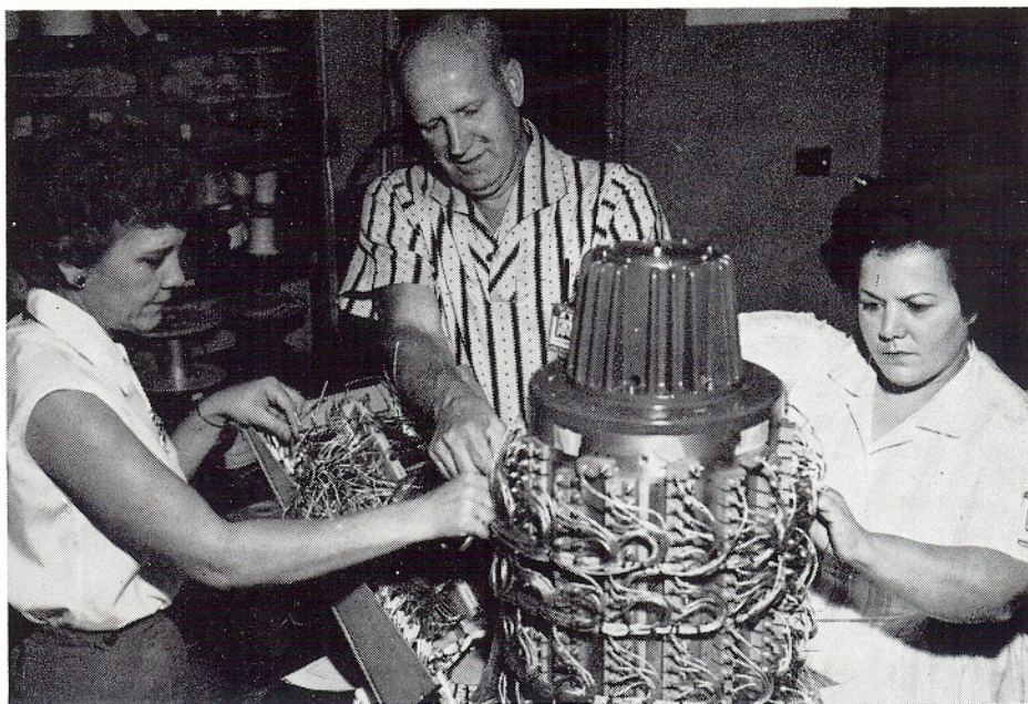
GLENDALÉ ASSEMBLY SECTION BUILDS MEMORY DRUM FOR RCA: Mrs. Iva Pate, Steve Jackman and Mrs. Ida Tripoli (l-r), production wiremen, work on huge memory drum built under subcontract from RCA. Glendale's machine shop milled the huge drum from an aluminum casting.
