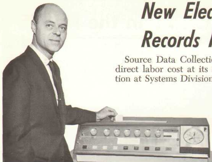
RECORDS LABOR COSTS — Pete Laue, senior industrial engineer, shows how the new Source Data Collection system records labor costs. "You merely insert a job data card into the Transacter and push the 'Transmit' button. Labor information is thus automatically recorded on tape at EDP."
