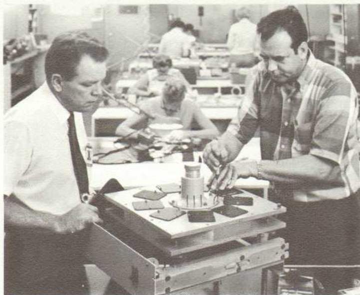
ASSEMBLY—Ed Ritts, Products Division assembler, right, installs one of the read/write heads on an L-416 Disc Memory as John Bennett, Industrial Engineer, looks on.
