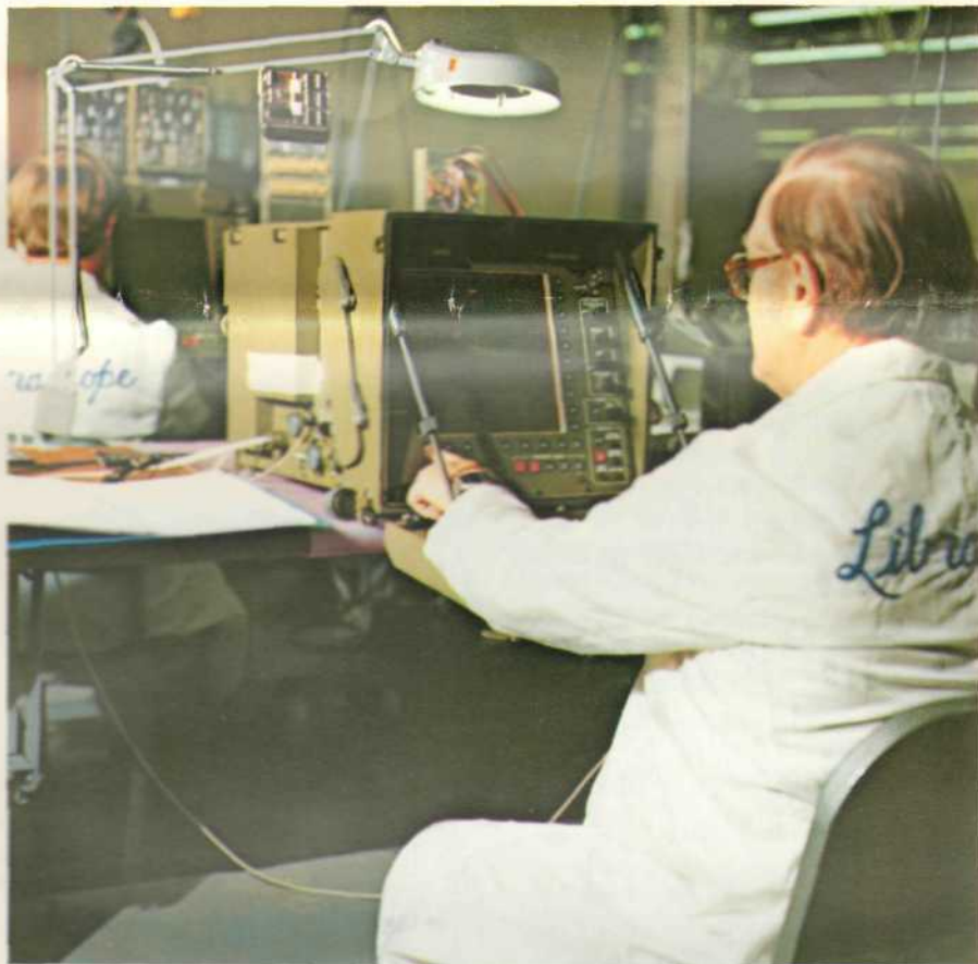
An E&M technician checks a TCT plasma panel, designed to provide the operator with electronic graphic tactical information, overlaid on a standard army paper map.
