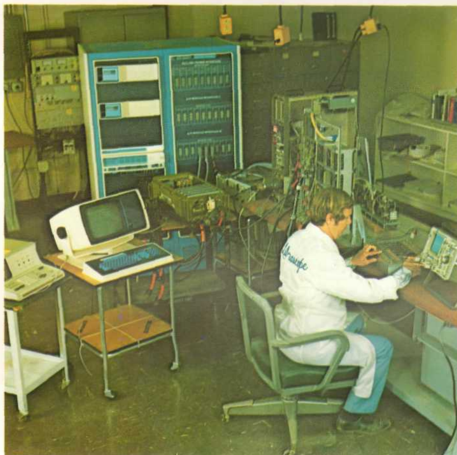
Testing of an I/O module is performed on Data General computerized test equipment. The I/O module is part of this year's program to provide ten (10) Tactical Computer Systems (TCS's) for the Army.
