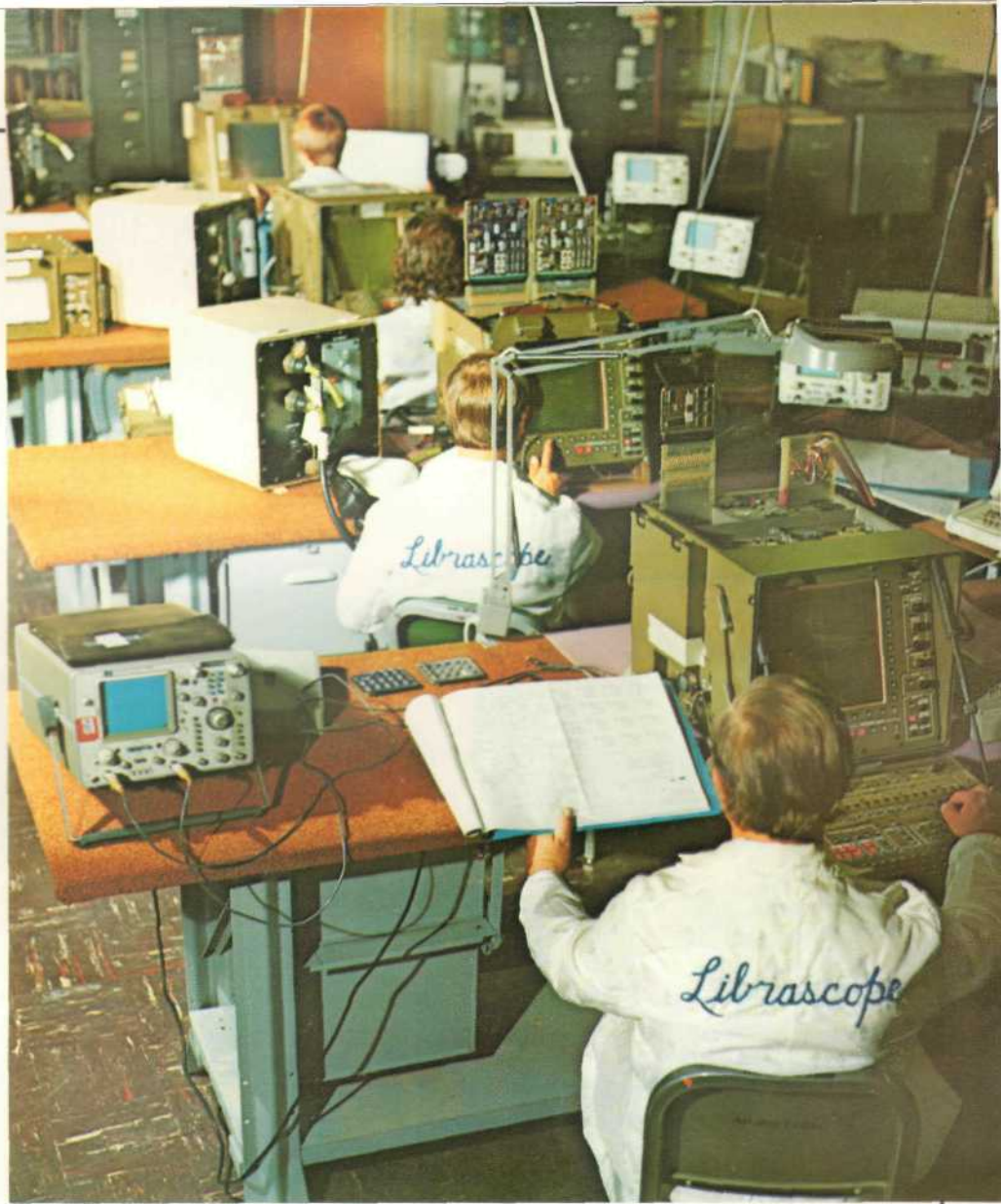
Librascope electrical/mechanical technicians perform final assembly and system checkout tests on Tactical Computer Terminals (TCT's). The equipment is being readied for use by the 7th Army in Germany.
