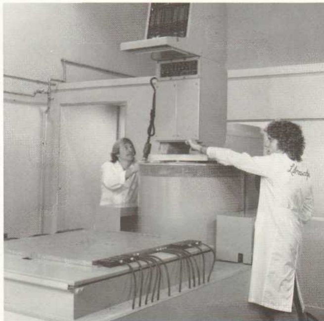
Test technicians, Eric Dodson (on right), and Scott Miller are shown securing an Attack Control Console, Mk 92, Mod 1, to the new 15,000 force pound Sine/Random vibration system.
