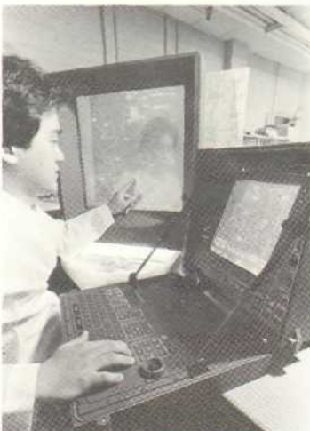
Librascope is a leader in employing plasma panels on militarized U.S. Army equipment. In the foreground is the TCT, with its 8 1/2 x 8 1/2 inch plasma panel, in the background is an auxiliary 17 x 17 inch panel.
