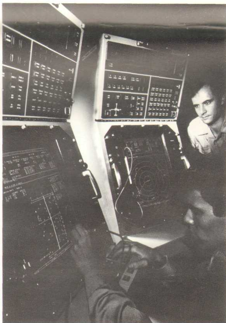
Librascope's Mk 1 highly-automated, underwater combat control system enables submarine personnel to perform threat analysis and weapon control functions on dual consoles. The Mk 1 is designed for international applications and has been purchased for installation on submarines of the Australian, Canadian and Indian navies. The photo shows a Canadian Mk 1 system in operation at Librascope.
