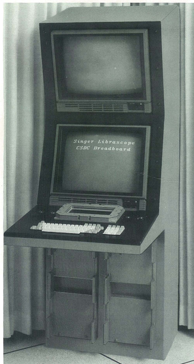
Librascope's breadboard design AN/BSY-2 Combat System Display Console (CSDC) for the U.S. Navy's next generation SSN-21 Seawolf Class submarines.
