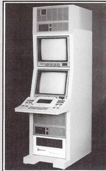
The Librascope-produced Imaging Center Console (ICC) is adapted from design concepts proven on the AN/BSY-2 Combat System Display Console, but modified to provide real-time video image processing.
