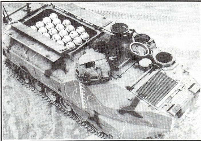
U.S. Marine Corps AAVP7A1-Mounted CATFAE System consists of a launcher, fuel-air explosive rounds, and fire control system components.
