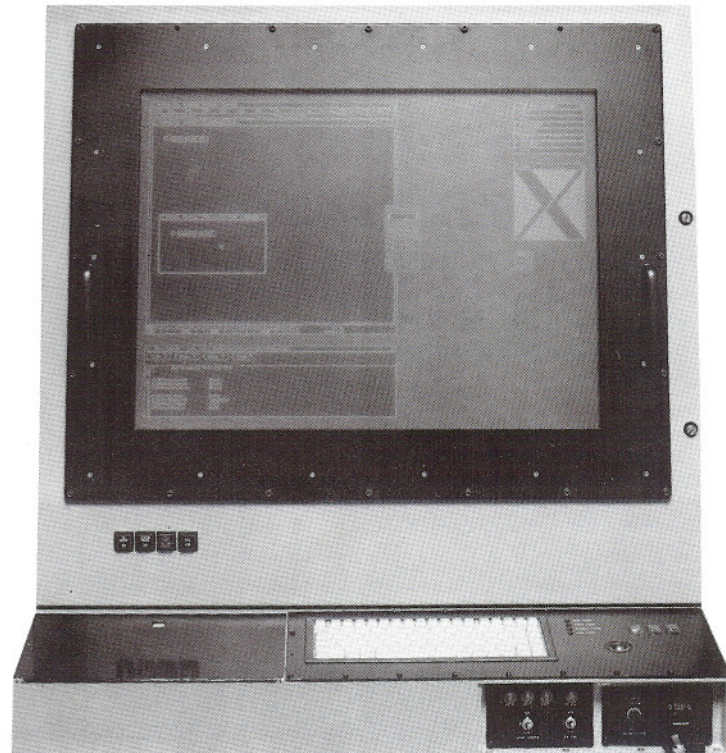
Command Display Console Submarine Fire Control System Mk 1
