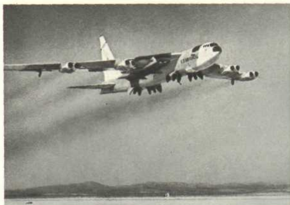
The pilot of the X-15 rocket ship will use GPL Doppler in a B-52 launching plane to calibrate and zero in his inertial guidance instruments.
