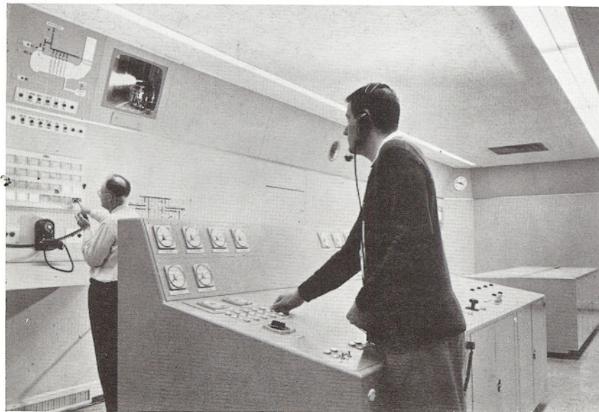
Engineer controls and analyzes rocket engine firing at flight propulsion laboratory by using GPL TV monitor.
