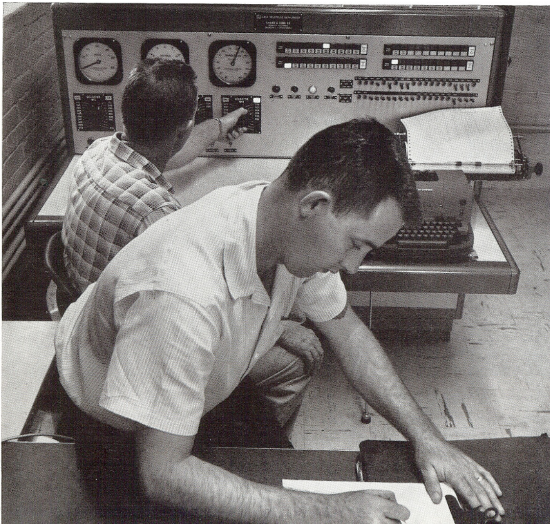
This Shand and Jurs Datalogger determines process variables such as storage tank levels and temperatures at a Richfield Oil Corporation marine terminal. Pilot lights signal high and low level alarms, and readings from a succession of tanks may be taken visually, or logged automatically on the electric typewriter.
