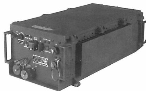
Magnetic Bubble Recorder Reproducer RD-509G (8 megabytes)
