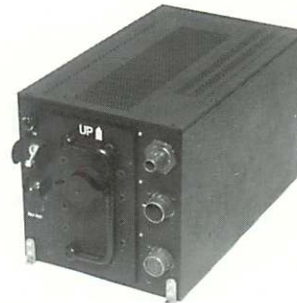
Mass Storage Device/Loader (2 megabytes)
