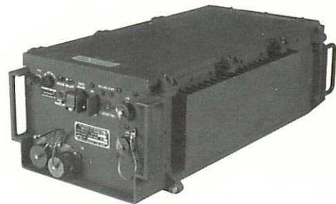
Magnetic Bubble Recorder Reproducer RD-509G (8 megabytes)
