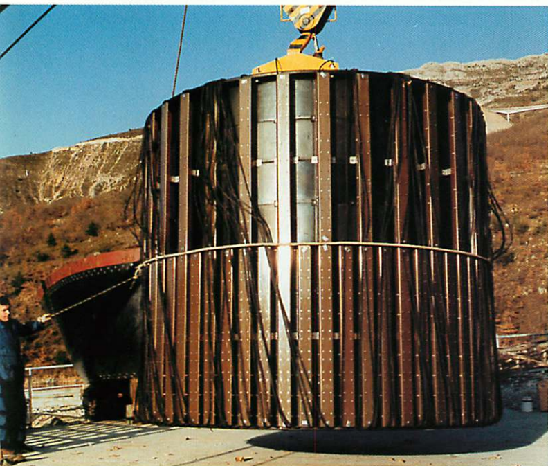
Search/Attack Array: Part of an integrated sonar system which provides detection and attack facilities
