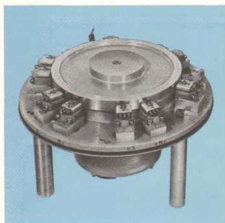
Memory drum turns at 3450 rpm
