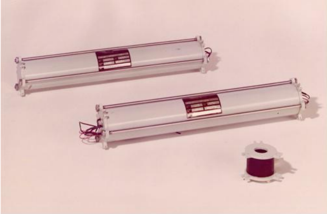
Figure 2 - One of the Singer Pinger Assemblies From top: Battery, Electronics, Transducer
