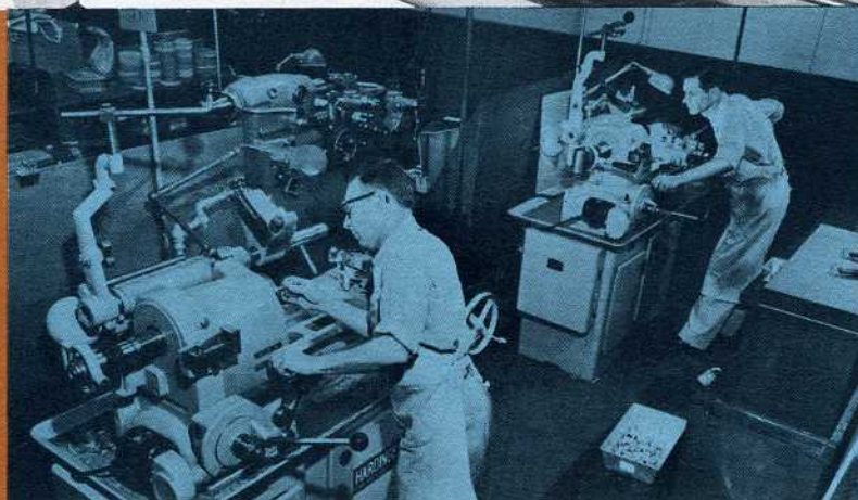
A Hardinge lathe, being used to ream the pen carriage bearing block castings for the Librascope X-Y Plotter
