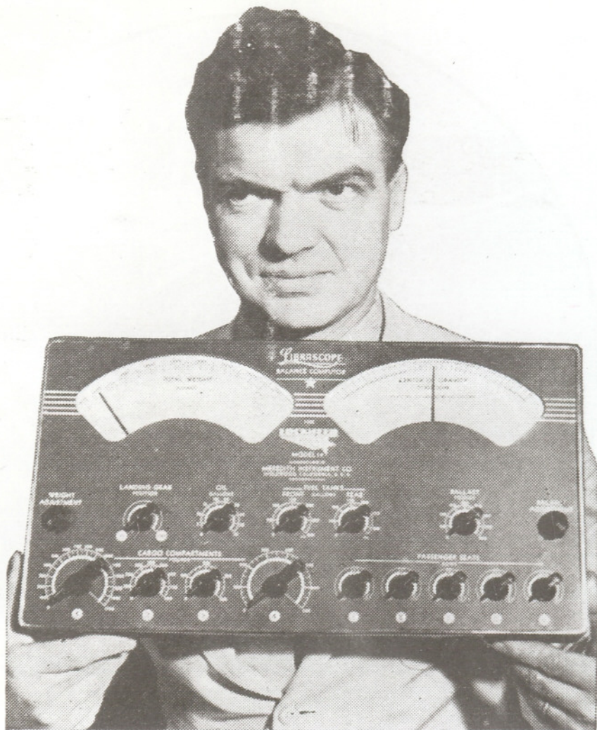
Holding the instrument board which shows which part of plane is heaviest
