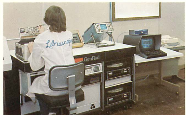
Technician conducting fault-finding of an Army PCB using AN/USM-105 automated test equipment
