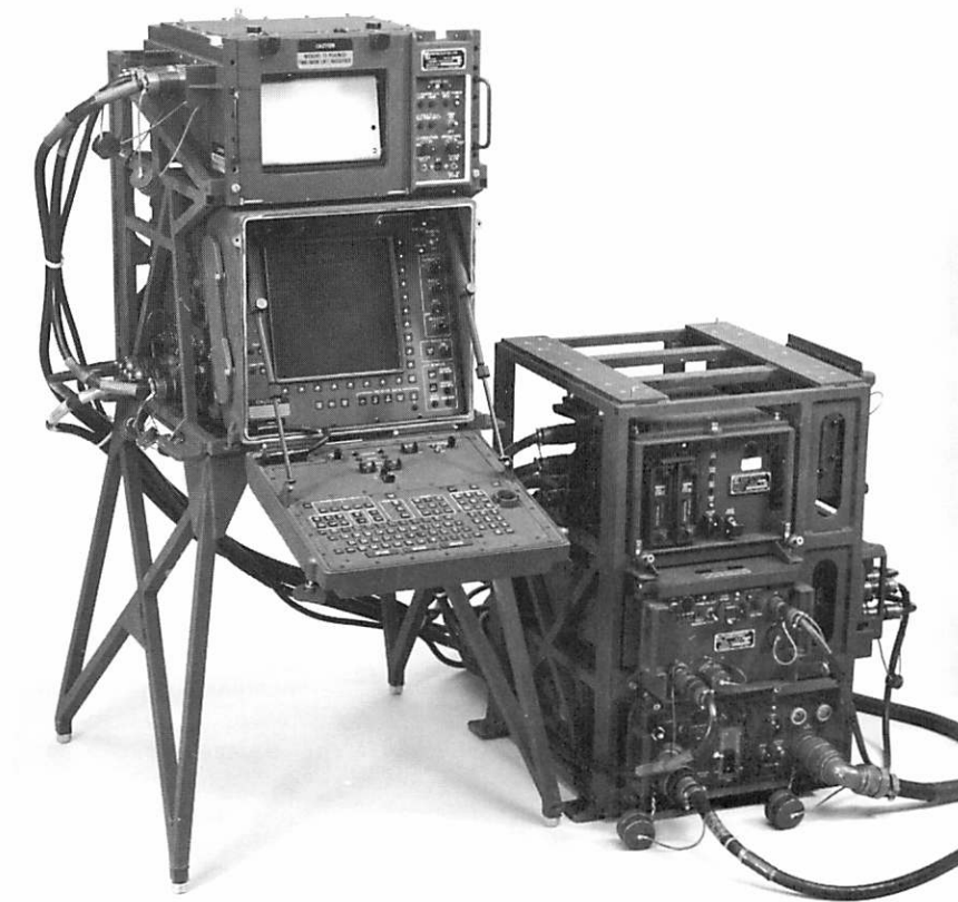
The tactical computer terminal (TCT) AN/UYO-30(A).
