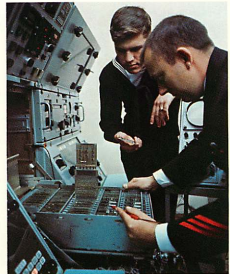
Ease of maintenance is an important feature of Librascope hardware. Control panel of Mk 113 console swings down to comfortable service position.
