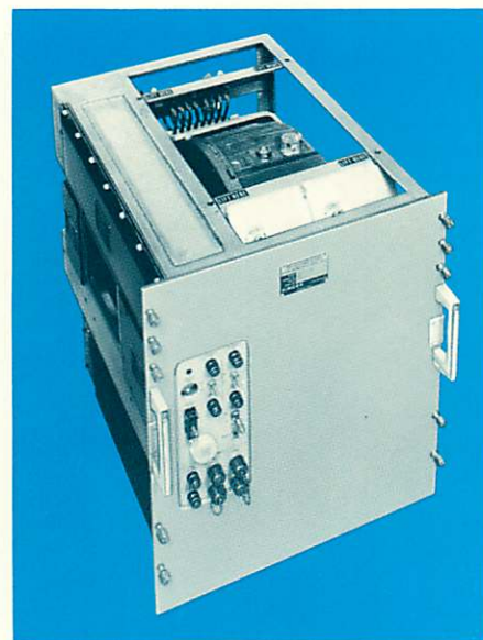
Librascope's Mass Memory Subsystem RD-433 is configured for Shipboard Tactical Intelligence (TACINTEL) Program. Meets full military specifications and it is EMI/RFI secure.
