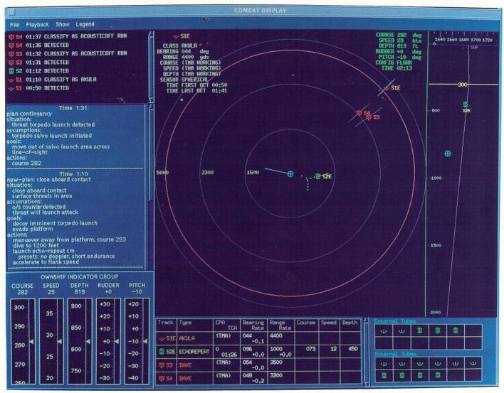
The Attack Response Mission Oriented Reasoner (ARMOR) is an automated decision aid that provides tactical advice to the command decision team of a submarine in case of torpedo attack. It is one of Librascope's Artificial Intelligence-based decision aids developed using the LINDA system.
