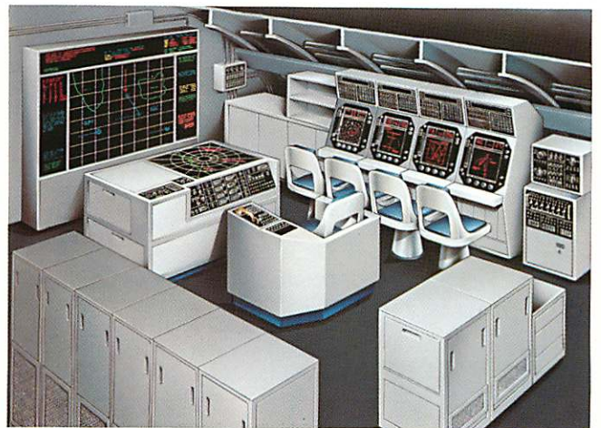
Displays can be vertical or horizontal, as shown in this depiction of a submarine combat systems center. Both graphic and alphanumeric data can be displayed simultaneously, in multiple colors.
