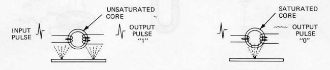
A simplified method of interrogating a magnetic encoder is to treat the sensor cores as in computer memory core matrixes. A single pulse interrogates the sensor cores to produce an output pulse for a "1", or none for "0".
