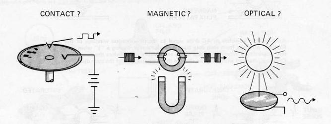
Digital encoders are electromechanical devices which translate input shaft angle information into digital electrical signals.
