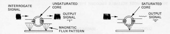
An oscillator furnishes an AC drive signal to the interrogation windings of the cores. Readout windings from each core transmit a signal representing a "1" when the core is not magnetically saturated, and a signal representing a "0" when the core is saturated. Cores are saturated when they are close to the magnetic areas of the code disc.
