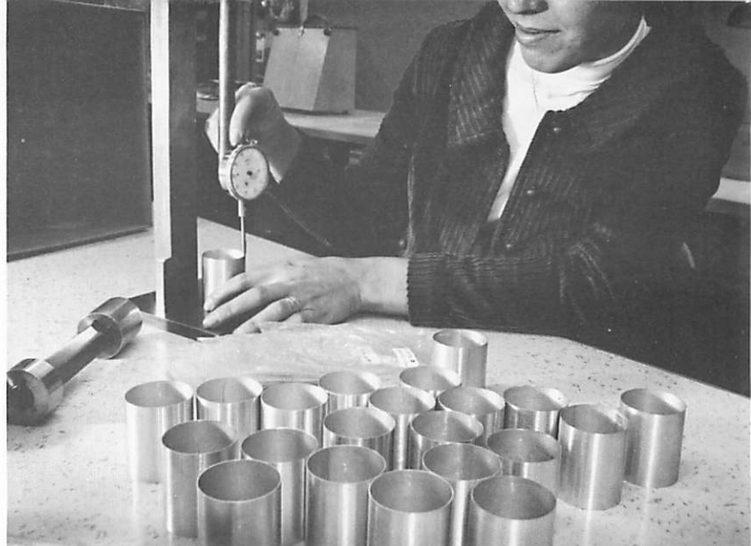
Another manufacturing step; Assembler checks and verifies dimensions of encoder covers with dial gauge.
