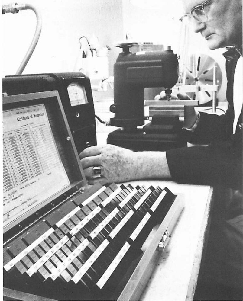
Engineer calibrates tools and gauges against "high-precision" reference blocks. This is but one of many procedures to assure precision fabrication of Librascope encoders.
