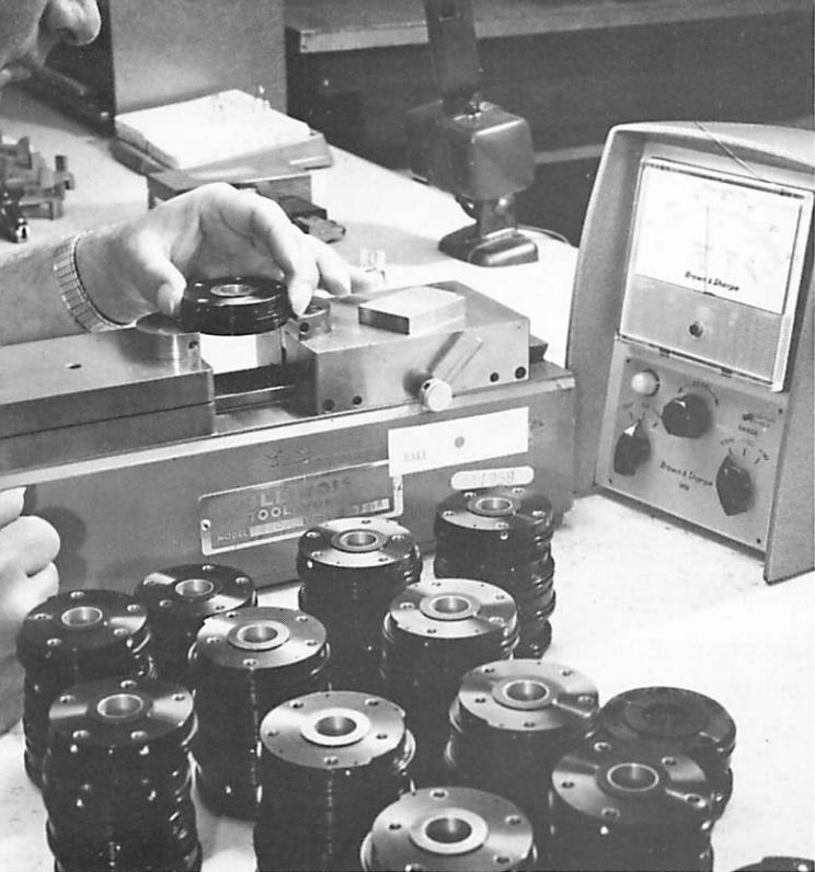
Frame fabrication; Technician using precise measuring equipment verifies diameter of encoder front frames.
