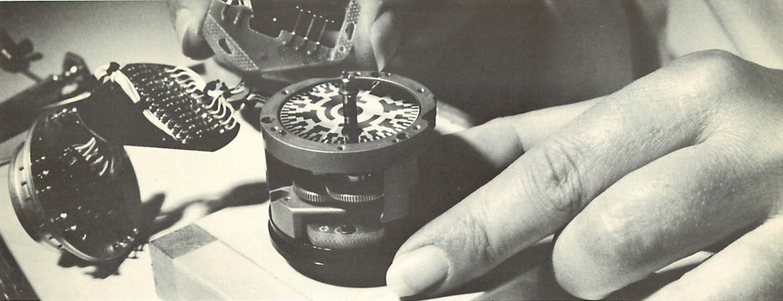
Encoder begins to assume final form as it nears end of assembly operation.
