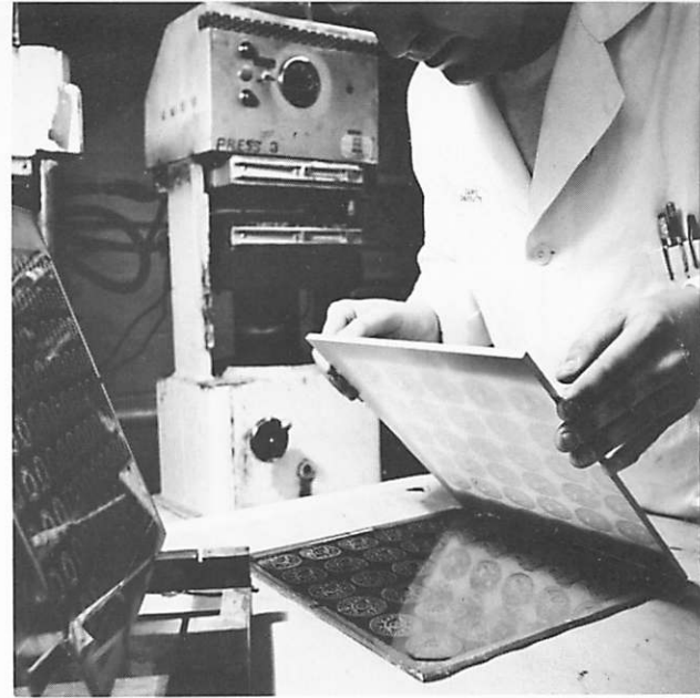
After gold plating, technician then strips plated images from plate, in preparation for curing process.
