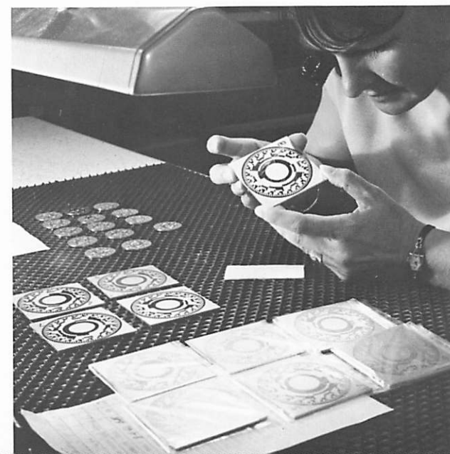
Discs are inspected again after cutting apart. Imperfect discs are discarded.
