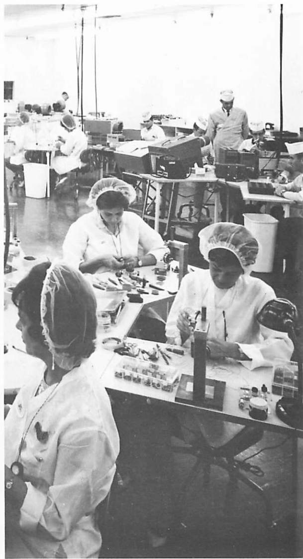
Technicians working at assembly operations in dust-free temperature-controlled assembly room.
