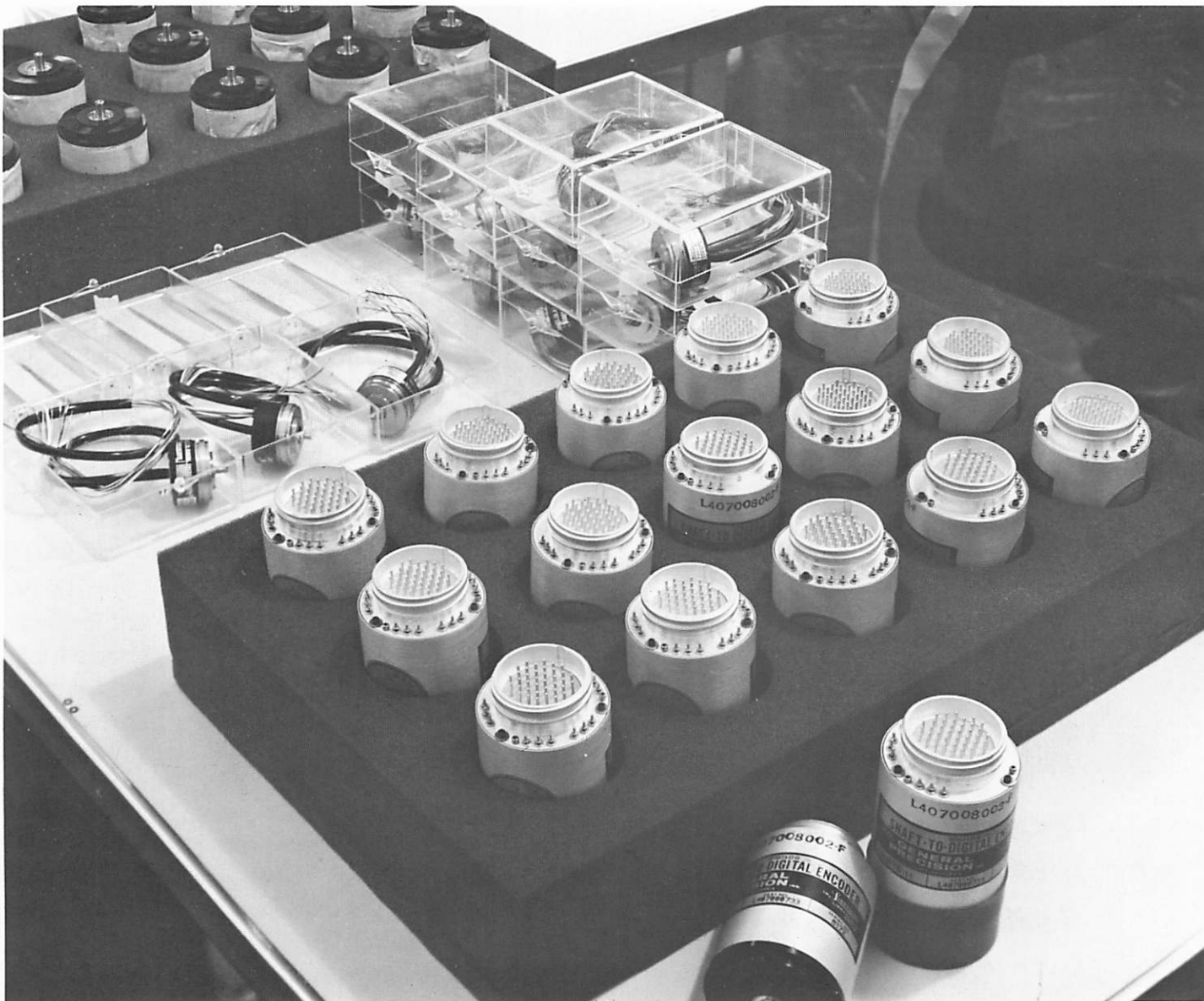
Work station in the assembly cycle. Encoders are taped for protection against dust contamination prior to final assembly.
