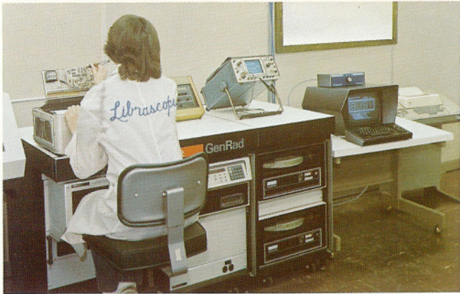
Technician conducting fault-finding of an Army PCB using AN/USM-105 automated test equipment
