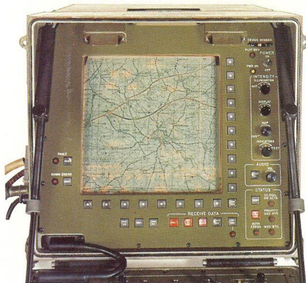
TCS Display showing data being superimposed on a map inserted behind the Plasma Panel
